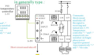
3. Single phase power regulator of VR type. Pure VR(JK01) wiring way.:
