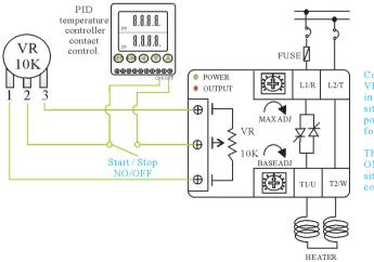
Comments VR has 3 feet, installs in 3 pieces of screw site of the Single phase power regulator VR type for 1, 2, 3 respectively.
