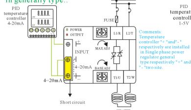
2. Single phase power regulator install the temperature controller 1-5V wiring way
