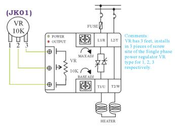
4. Single phase power regulator VR type, pure VR and install temperature controller contact control (ON-OFF) the wiring way.:
