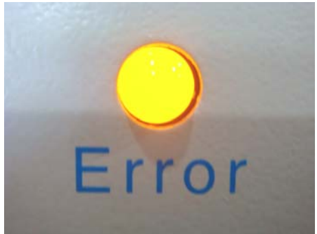
Light ON, and glimmered as 5 phases when error happened.
