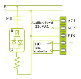
Three phases power used in SCR products. Suggest control wiring diagram.
